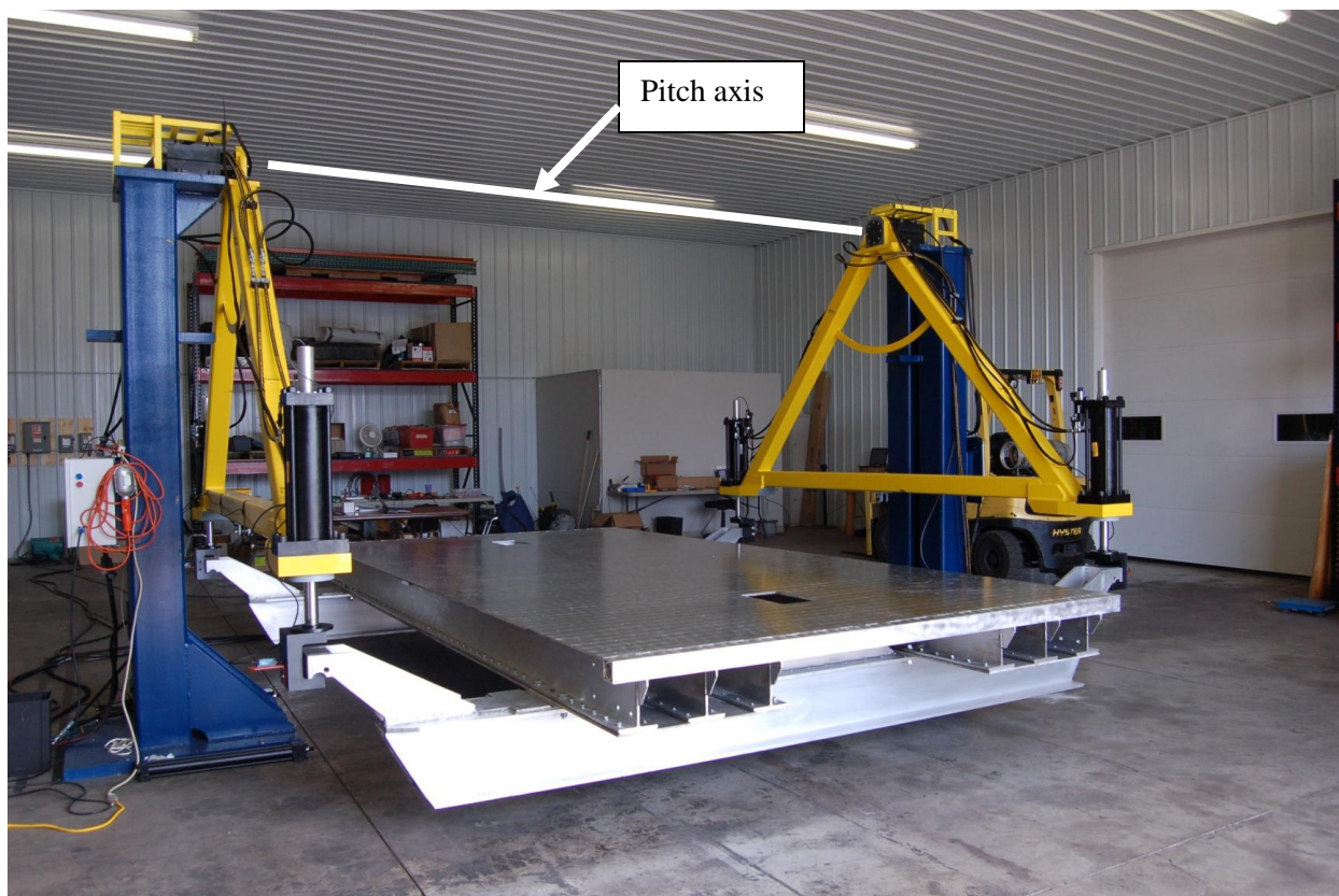
Figure 1: The small platform (aluminum) fixed pylons (blue) and swing arms (yellow).
